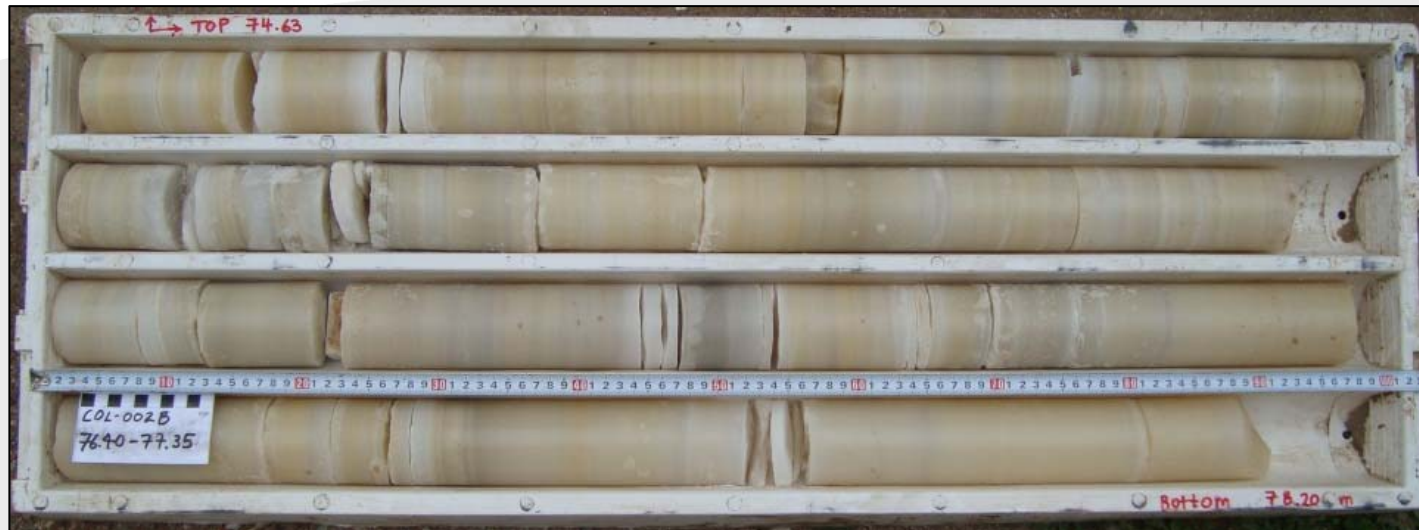
Above; COL-002B drill core showing the base of a strong carnallite zone from 63.25 – 67.00m. Below; COL-002B drill core showing kainite zone from 74.63 – 78.20m.
