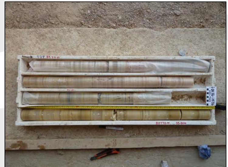
COL-001 drill core showing base of a strong carnallite mineralisation zone from 89.74 - 93.20m (note carnallite is heat sealed in plastic immediately after drilling to prevent dissolution of the samples)
