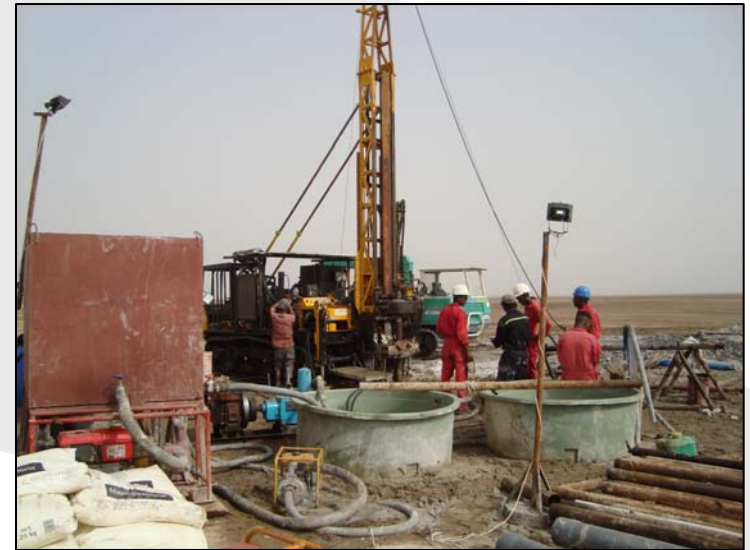
South Boulder Drill Crew conducting the second diamond hole at The Colluli Potash Project, Eritrea.
