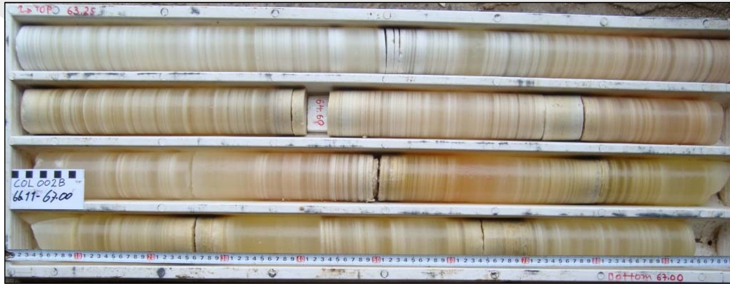
Above; COL-002B drill core showing the base of a strong carnallite zone from 63.25 – 67.00m. Below; COL-002B drill core showing kainite zone from 74.63 – 78.20m.
