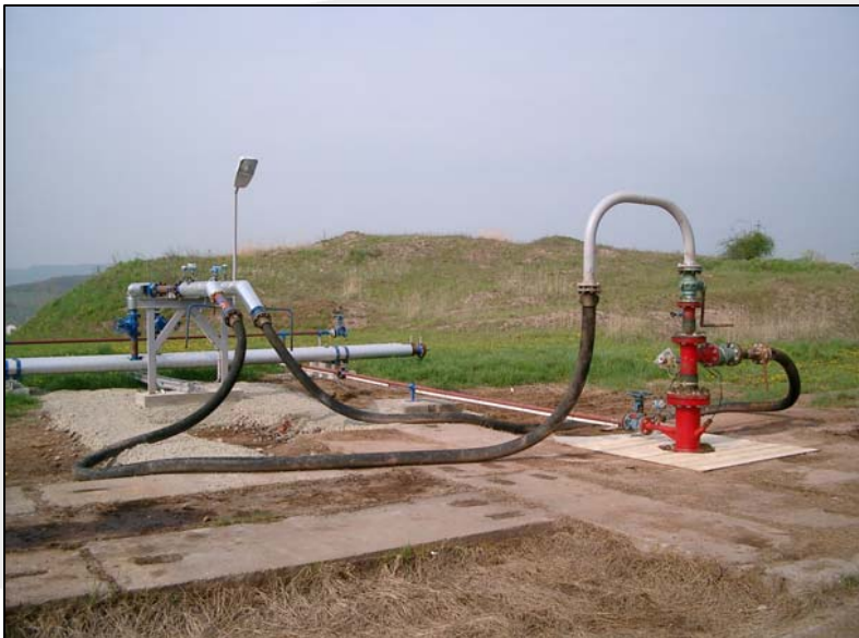
Above; Viscosity testing of diamond drilling mud for good recovery of the potash zones. Below; A typical solution mine well head and distributor.
