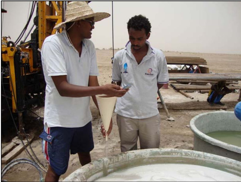
Above; Viscosity testing of diamond drilling mud for good recovery of the potash zones. Below; A typical solution mine well head and distributor.
