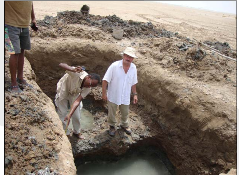
Above; Drill sumps in the salt flat provide a source of drilling water. Below; Carnallite zone drill hole COL-002B ( \text{KMgCl}_3 \cdot 6(\text{H}_2\text{O}) ).
