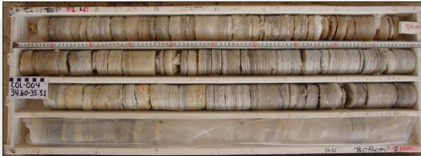
Above; COL-002B drill core showing the base of a strong carnallite zone from 63.25 – 67.00m. Below; COL-004 drill core showing strong sylvinite zone from 34.60 – 35.51m.
