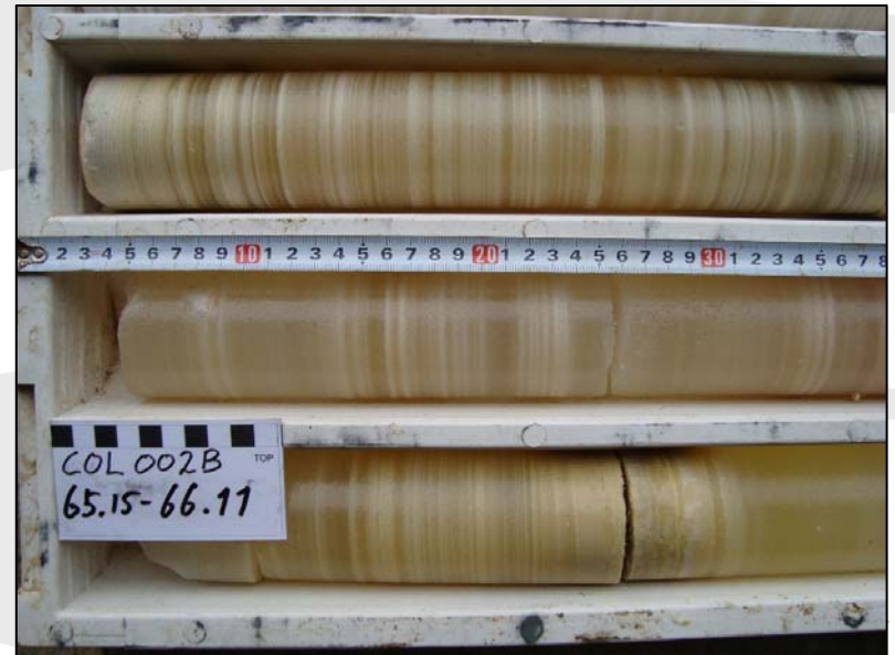
Above; Drill sumps in the salt flat provide a source of drilling water. Below; Carnallite zone drill hole COL-002B ( \text{KMgCl}_3 \cdot 6(\text{H}_2\text{O}) ).
