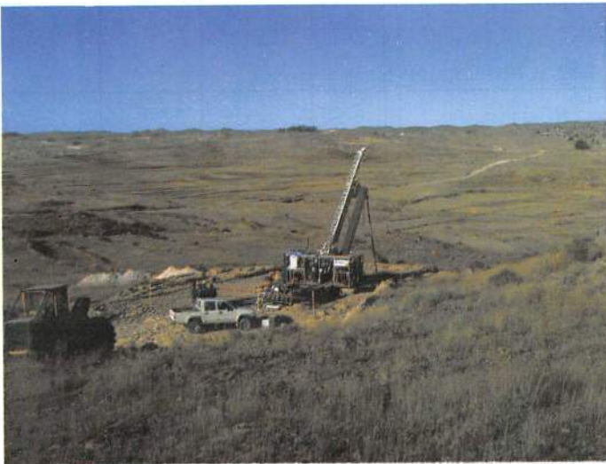
Core drilling at Emba Derho
